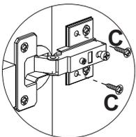
**detalhe 10****10 FIXAÇÃO NA PAREDE**
